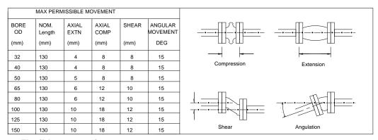
Fig. 1.2 Flexible connections
