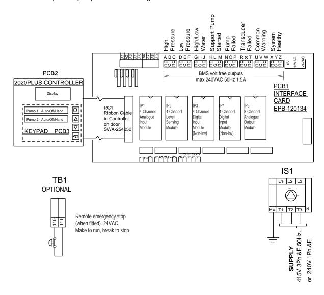
Fig. 1.3 Typical example of electrical connections
