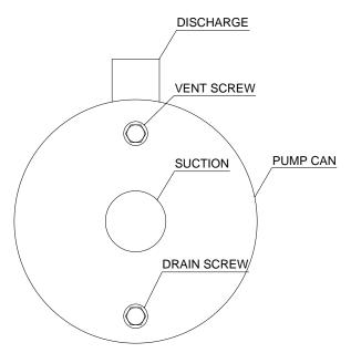
Fig 2.1 Venting Pumps (Multi-Stage type pump shown above, End-Suction type pump below)
