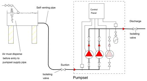
Fig. 1.1 Typical Pipework arrangement
